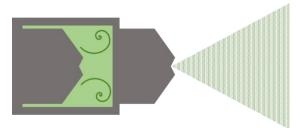
Figure: example of a double chamber and the flow within it.
