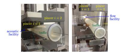
Fig. 1. Prototype of upper airway replica with a simplified timevarying waveguide set in a baffle. Both acoustic (left) as flow (right) fields are studied.
