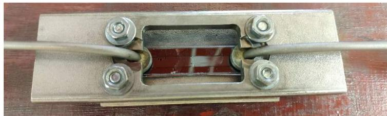
Prototype of the microfluidic system
